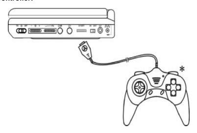
**\*Note:** Do not use the "AV Jack" and "E Port" at the same time when in "AV IN" mode. Unplug the game controller when using the A/V input jack.
